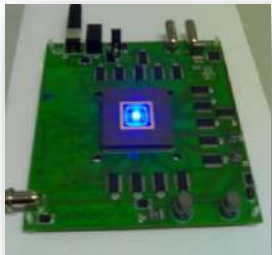
64x64, 64x1 passive μLED arrays
